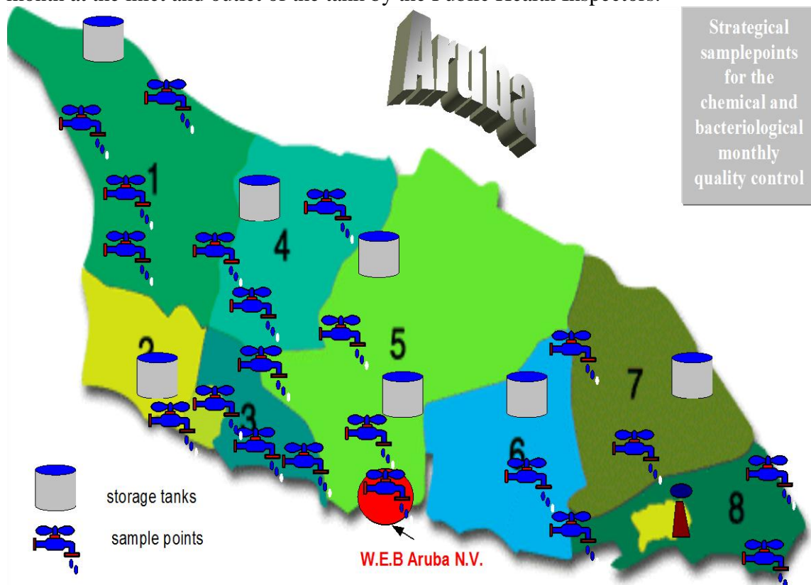
Figure 12:Storage tanks and samplepoints in the distributionsystem.
